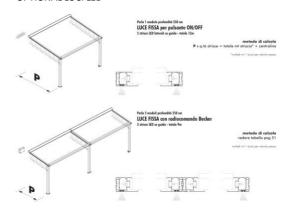
DIMENSIONI MASSIME A MODULO IN LARGHEZZA Metri 5 DIMENSIONI MASSIME A MODULO IN SPORGENZA Metri 6
